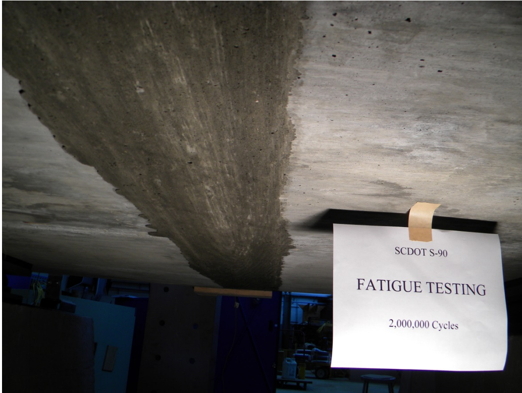
Figure 3.23: Underside of joint after fatigue loading
